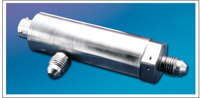
The Kulite BMD/BMDE-1100 Series pressure transducers are designed for the measurement of pressure drop across air and oil filters, engine torque and similar applications. Available either unamplified (100mV output) or amplified (5 volt output), these units are all stainless steel construction with weld sealing offering maximum accuracy and performance for industrial and aircraft applications.
