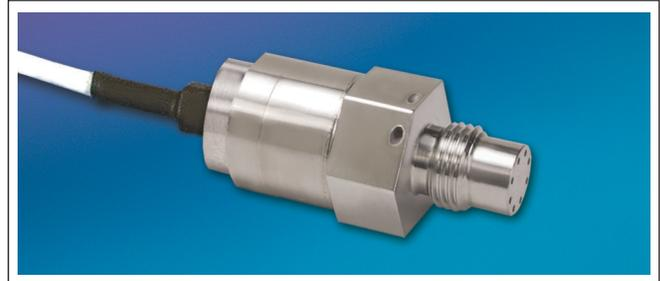
ETM-375 series transducers are miniature, threaded flush diaphragm instruments. They utilize a flush metal diaphragm as a force collector. Force is transferred to a solid state piezoresistive sensing element via a thin intervening film of non-compressible silicone oil. This sensing sub-assembly is protected from mechanical damage by a solid screen
