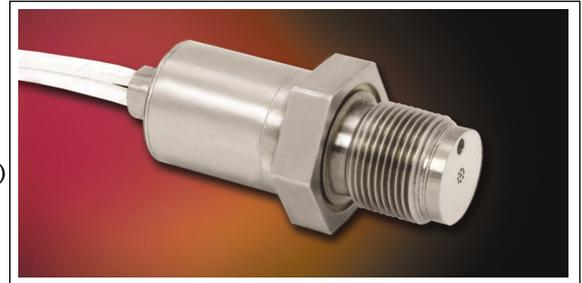
The XTEL-5-SD-625 (Inconel) Series are high temperature extremely rugged pressure transducers which are ideal for the measurement of flow instabilities and steady pressures in gas turbine combustors and compressors. The XTEL-5-SD-625 (Inconel) uses an innovative low-pass mechanical filter to enable the measurement of low-level dynamic pressures in high pressure environments with superior
